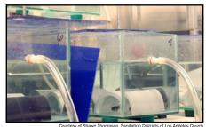
During traditional toxicity testing, organisms such as fish are exposed to water samples in a laboratory. Bioanalytical screening has the potential to reduce reliance on wholeorganism toxicity tests.
