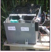
Fish that have been placed in mobile exposure units, above, are exposed to flowing Los Angeles River water in real time. Researchers are tracking whether fish are impacted by CECs in the water.
