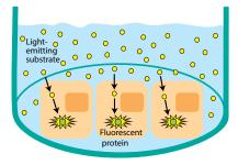
The strength of the signal reflects the CEC levels in the water sample.
