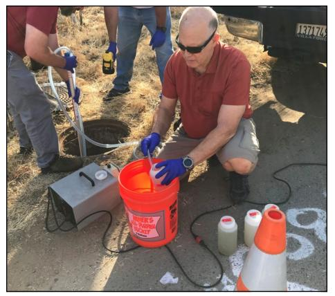
SCCWRP's Dr. John Griffith uses a peristaltic pump to vacuum contents from an underground sewer pipe in San Diego County. Researchers are investigating whether the microbial community that lives inside the pipes – known as biofilm – is distinguishable from the biofilm in storm drain pipes, which could help narrow down the origins of widespread fecal contamination in Southern California waterways during wet weather.
