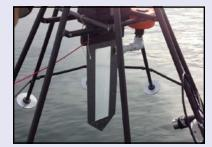
A field crew deploys a passive sampling device into San Diego Bay for a study probing the origins of contamination found in fish in the bay. The device consists of a pointed metal frame containing polyethylene film that is inserted into seafloor sediment.
