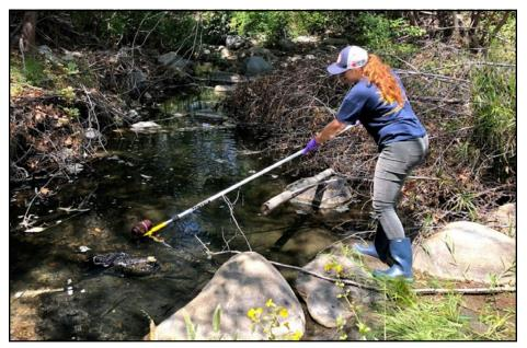
SCCWRP's Dana Shultz collects a water sample in Upper San Juan Creek in San Diego County just a few feet from where mussels in metal cages have been temporarily placed into the stream. Researchers are investigating the feasibility of identifying organisms by the DNA they shed into their environment, known as environmental DNA.
