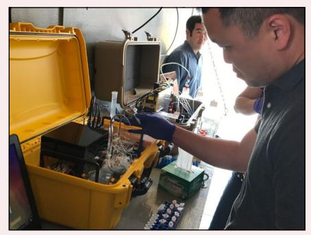
SCCWRP's member agencies test a suitcase-sized, portable instrument that could help track fecal contamination to upstream points of origin. The device was tested in a SCCWRP mobile laboratory.
