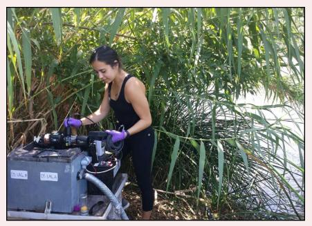
SCCWRP's Syd Kotar monitors water quality inside a mobile unit that houses fish. The units, set up along the banks of the Los Angeles River, were used to expose the fish to flowing river water in real time, enabling researchers to track potential biological impacts from exposure.
