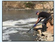
SCCWRP's Dr. Amy Zimmer-Faust collects a water sample at the site where Mexico's San Antonio de Los Buenos treatment plant discharges primarytreated effluent into the coastal ocean. Researchers are examining whether fecal contamination at this site is traveling north to Imperial Beach near the U.S.-Mexico border.
