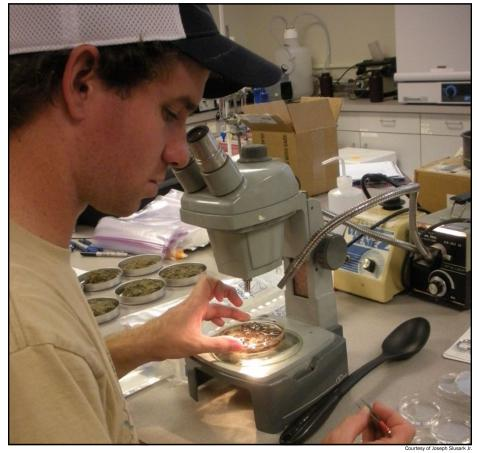
Insects and other benthic macroinvertebrates are removed individually with tweezers from a streambed sample so they can be counted and identified under a microscope. Scientists are exploring ways to identify these organisms using DNA sequencing methods.
