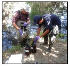
A SCCWRP field crew collects water samples to screen water bodies for chemical contaminants using multiple laboratory methods, including bioanalytical screening.
